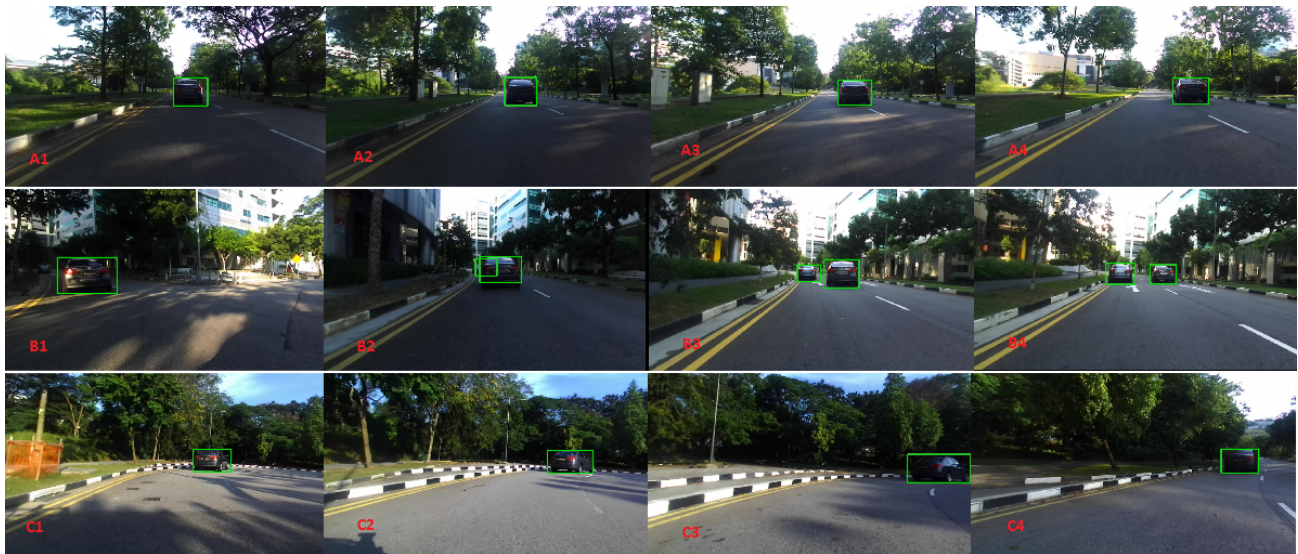
Fig. 11. A: Selected image sequences showing the target vehicle performed lane changing in a straight two-lanes road. B: Selected image sequences showing the target vehicle overtaking a parked vehicle. C: Selected image sequences showing the target vehicle making a 90^\circ turn.
